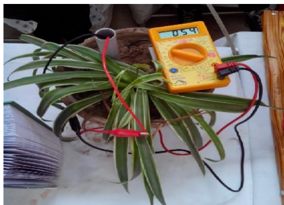
Fig. 1: Experimental set of P-MFC.
